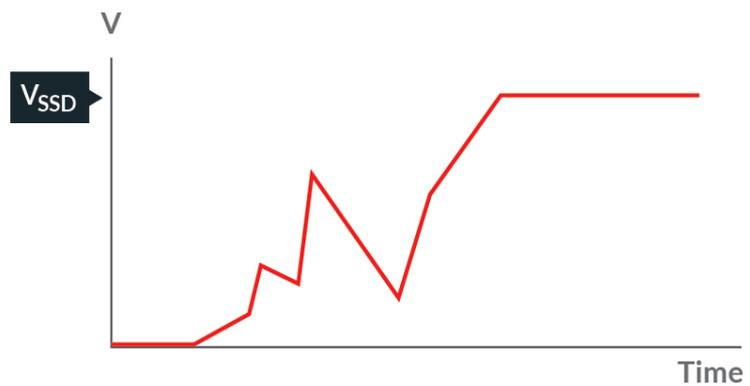
Graph 2: Fluctuating voltage during SSD ramp-up.
