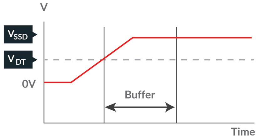
Graph 3: After reaching the threshold voltage ( $V_{DT}$ ), the SSD adds a buffer zone to ensure that it achieves stable voltage ( $V_{SSD}$ ) before initiating a startup.
