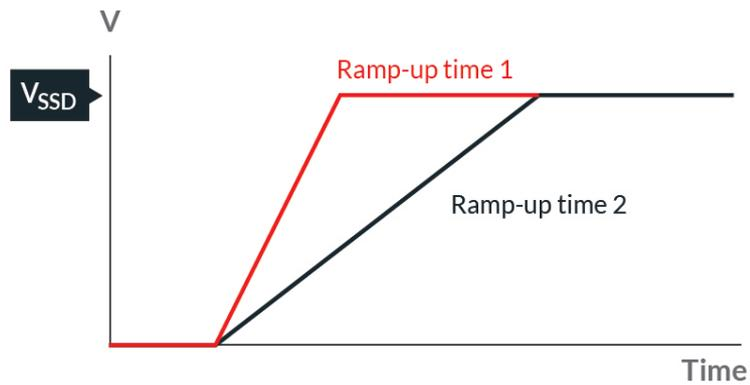
Graph 1: Two examples of differing device ramp-up times.
